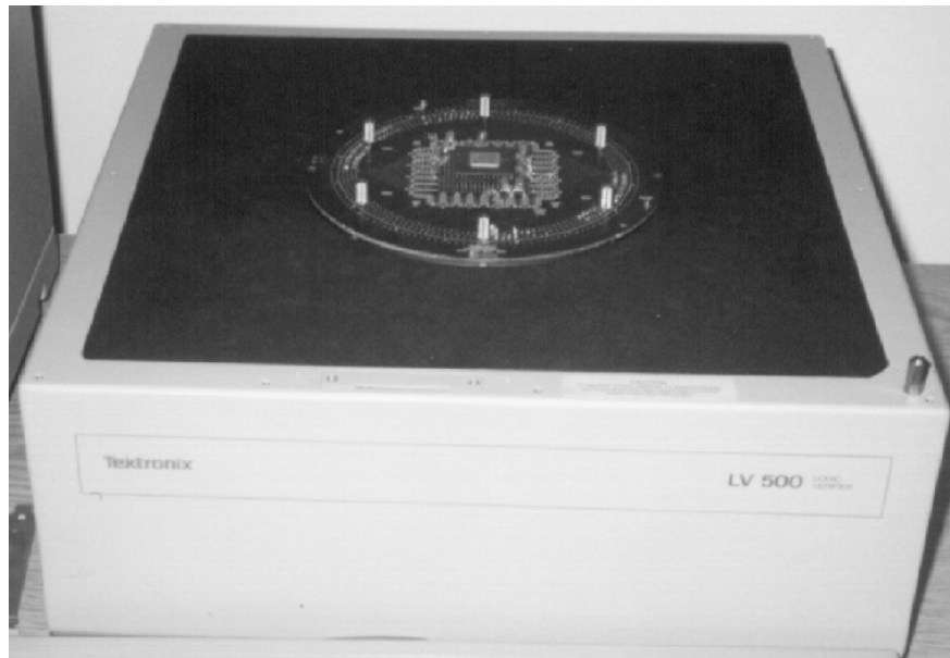
Figure 6: The LV500 Test Jig with the FM9001
