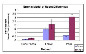
Figure 7 – Error in models of the differences between the two robots, when using instances obtained while establishing a physically shared context using the three methods.
