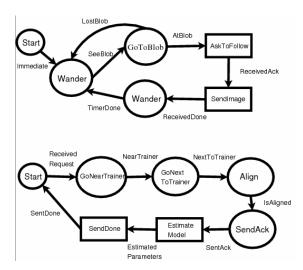
Figure 3 - FSA for the "follow" method. On the top is the trainer FSA and on the bottom is the learner FSA.
