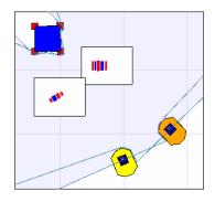
Figure 1 – Left: Map of the environment, corresponding to the layout of the robot laboratory. Right: Zoom in of robots, showing the object (upper left), two robots, and their points of view in the blob finder (squares). Note the differences in scale (due to the zoom of the camera) and camera angle.
