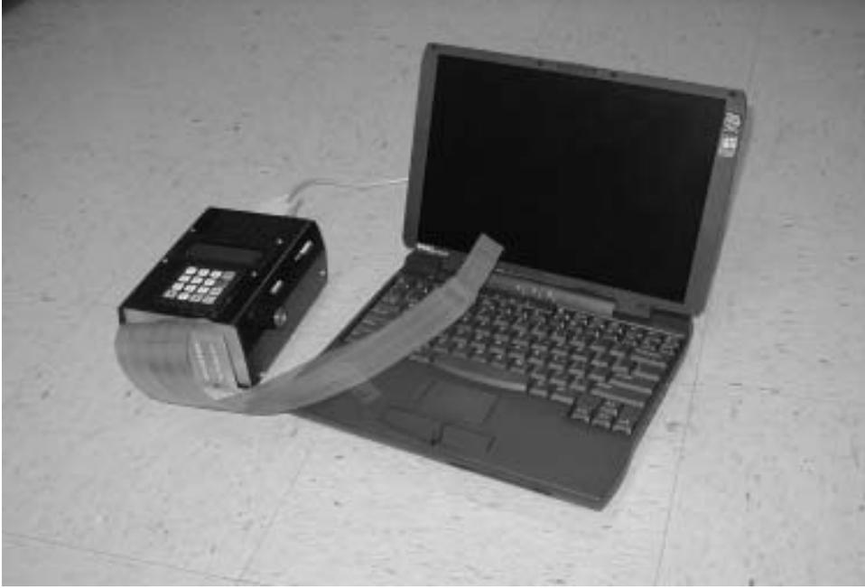
**FIGURE 2** TDU-1 with 144-point tongue array & laptop PC.
