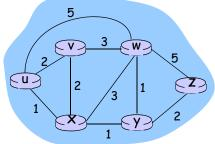
$$\begin{aligned} d_{u}(z) &= \min \big\{ \ c(u,v) + d_{v}(z), \\ c(u,x) + d_{x}(z), \\ c(u,w) + d_{w}(z) \big\} \\ &= \min \big\{ 2 + 5, \\ 1 + 3, \\ 5 + 3 \big\} = 4 \end{aligned}$$
