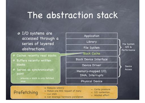
The abstraction stack Application accessed through a Library series of layered File System API & File System abstractions Performance Block Cache **Block Device Interface** Device Driver Device written in fixed-sized blocks Access Memory-mapped I/O, Output Uniform interface to DMA, Interrupts disparate devices **Physical Device**
