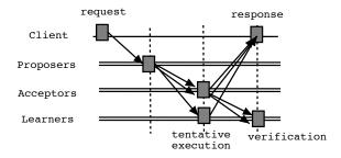
Figure 3. FaB state machine with tentative execution.
