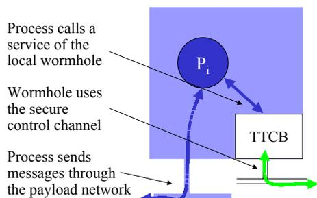
**Figure 1. Architecture of one node (the payload system is represented in dark and the wormhole in white).**
