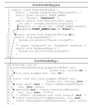
Figure 1. Example bug: a typo in Java code (line 15) causes a crash in C code (line 31).
