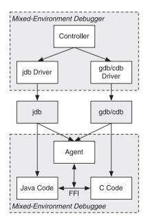
Figure 2. Agent-based debugger composition approach.
