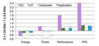
(d) Memory bandwidth effect. The high memory bandwidth is  $1.33\,\mathrm{GHz}$  x 2 channels relative to  $0.8\,\mathrm{GHz}$  x 1 channel.
