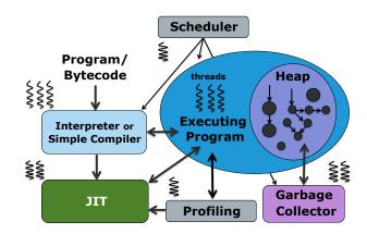
Fig. 2. Basic Virtual Machine services and structure
