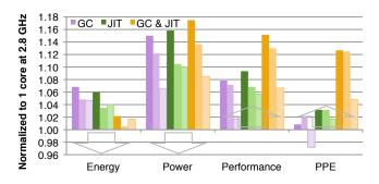
Fig. 5. Utility of adding a core dedicated to VM services on total energy, power, time, and PPE. Overall effect of binding GC, JIT, and both GC & JIT to the second core running at 2.8 GHz (dark), 2.2 GHz (middle), and 0.8 GHz (light) on the AMD Phenom II corrected for static power. The baseline uses one 2.8 GHz core.
