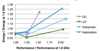
(c) Effect of clock frequency on performance and energy. Points are clock speeds 1.6, 2.0 and 3.4 GHz (from left to right) on i7 4C2T.
