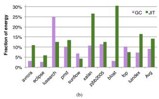
Fig. 4. GC, JIT, and application power and energy on i7 4C2T at 3.4 GHz. (a) Average power for GC, JIT, and application. (b) Fraction of energy due to GC and JIT. The power demands of the GC and JIT are relatively uniform across benchmarks. Together they contribute about 20% to total energy.
