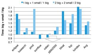
(b) Execution time increase due to adding small cores on an AMD Phenom II.  $^{1}$
