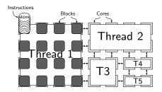
Figure 1. Mapping blocks to composable TFlex cores.
