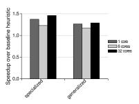
Figure 7. Speedup of learned heuristics on microbenchmarks normalized to the baseline heuristic at the same core count.
