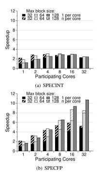
Figure 5. Performance with 128 instructions per core and fixed-size blocks. Thus, with maximum block sizes of 32, 64, and 128 instructions, there are 4, 2, and 1 blocks per core, respectively, and all configurations require the same number of issue queue slots.
