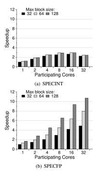
Figure 4. Performance with one fixed-size block per core and maximum fixed block size of 32, 64, and 128 instructions. Fewer hardware resources are required with smaller maximum block sizes.
