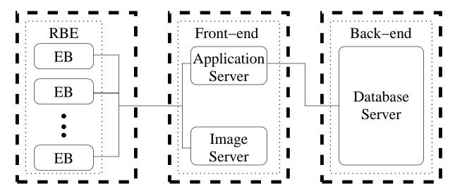
Figure 1. The 3 machines used in the physical setup. The thick, dashed rectangles represent physical machines. The dotted rectangles are processes, and the innermost rounded rectangles are logical units. Network connections are shown as lines and come together at the point where they are managed; i.e., Tomcat handles routing of connections to the application and image servers, while the physical machine coalesces the individual EBs' network connections.
