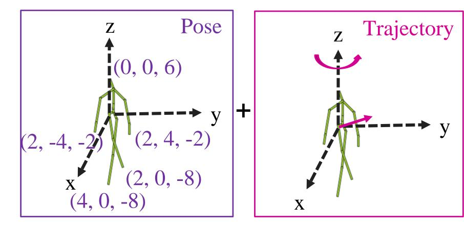
Figure 2: (Left) The character's pose is represented by the joint positions in the local coordinate frame. (Right) The character's trajectory is represented by the rotational velocity about the z-axis and translational velocity on the yz-plane.
