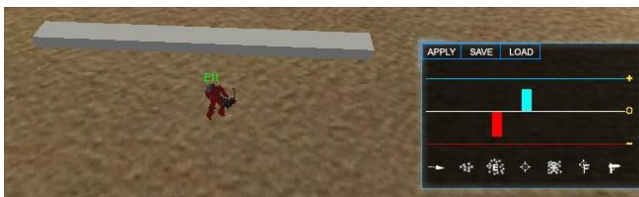
Figure 6: Setting up training scenarios (color figure). This screenshot shows items the player can place on the field and sliders used to control behavior. The red robot is a stationary enemy turret that turns back and forth as it shoots repetitively. Behind the turret is a wall. The player can place turrets, other kinds of enemies, and walls anywhere on the training field. On the right is the box containing slider controls. These sliders specify the player's preference for the behavior the team should try to optimize. For example the "E" icon means "approach enemy," and the red bar specifies that the player wants to punish robots that approach the enemy. The crosshair icon represents "hit target," which is being rewarded. The sliders represent fitness components that are used by rtNEAT. The value of the slider is used by rtNEAT as the coefficient of the corresponding fitness component. Through placing items on the field and setting sliders, the player creates training scenarios where learning takes place.
