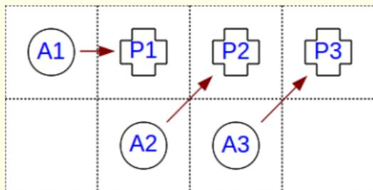
Lowest lexicographical cost (shown with arrows) to highest cost ordering of mappings from agents (A1,A2,A3) to role positions (P1,P2,P3). Each row represents the cost of a single mapping.
