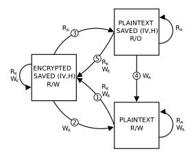
Figure 1. Basic Cloaking Protocol. State transition diagram for maintaining the secrecy and integrity of a single cloaked page. Application reads  $R_A$  and writes  $W_A$  manipulate plaintext page contents, while kernel reads  $R_K$  and writes  $W_K$  use an encrypted version of the page. A secure hash H is computed and stored immediately after page encryption, and verified immediately prior to page decryption.
