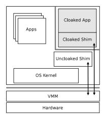
**Figure 2. Overshadow Architecture.** The VMM enforces two virtualization barriers (gray lines). One isolates the guest from the host, and the other cryptographically isolates cloaked applications from the guest OS. The shim cooperates with the VMM to interpose on all control flow between the cloaked application and OS.
