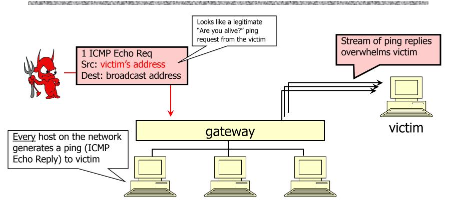
Solution: reject external packets to broadcast addresses
