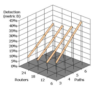
Figure 2: Metric B: probability of observing the true initiator at least twice  $(\frac{1}{6} \text{ of routers are corrupt})$
