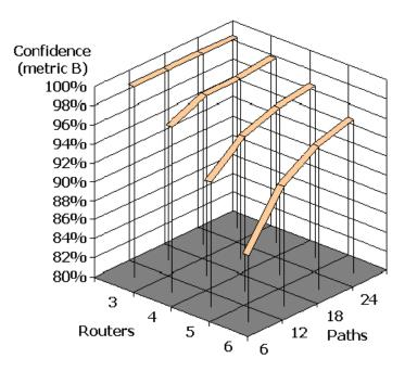
Figure 3: Metric B: probability of observing <u>only</u> the true initiator at least twice  $(\frac{1}{6}$  of routers are corrupt)
