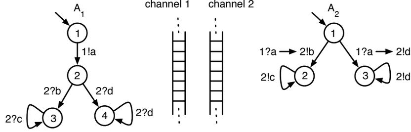
Fig. 4. An example of a FIFO system consisting of two processes and two channels.
