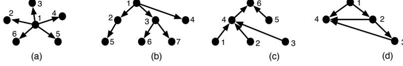
Fig. 9. Communication topologies: (a) star, (b) tree, (c) inverted tree, (d) DAG.
