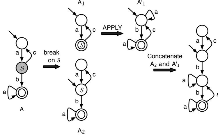
Fig. 8. An example illustrating PREFIX operation with automaton  $A$ , state  $s$ , and  $Act = \{?a \rightarrow !b, ?b \rightarrow !a, ?c, !a\}$  as inputs.
