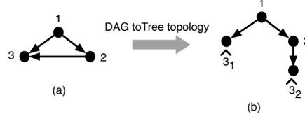
Fig. 14. (a) DAG communication topology, (b) Converting DAG to inverted tree using shadow channels.
