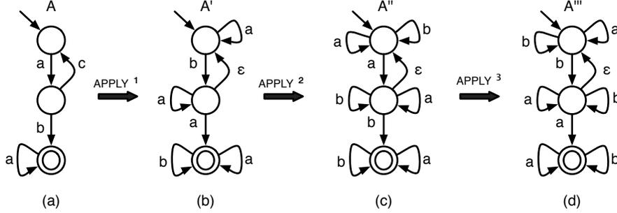
Fig. 7. An example illustrating PHASE1 with automaton  $A$  and  $Act = \{?a \rightarrow!b, ?b \rightarrow!a, ?c, !a\}$  as inputs.
