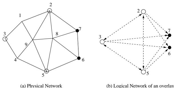
**Figure 1: A physical network and the logical network for the overlay formed by nodes 2, 3, and 5. Nodes 6 and 7 are not overlay nodes but nodes 2, 3, and 5 have demands to them. The logical link from node 2 to 5 consists of two physical paths: 2 to 9 to 5, and 2 to 8 to 5, if hop-count OSPF routing is used.**
