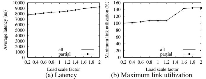
Figure 10: Effects of partial coverage on the performance of selfish overlay routing. Here edge nodes in *ISPT<sub>opo</sub>* belong to an overlay, and OSPF weights are set according to hop count.
