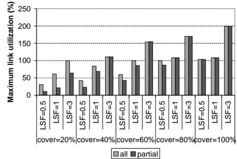
Figure 11: Effects of partial coverage in *ISPT<sub>opo</sub>* with random node selection on maximum link utilization.
