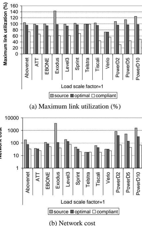
Figure 6: Selfish source routing: comparison of maximum link utilization and network cost using M/M/1 link latency across different network topologies.
