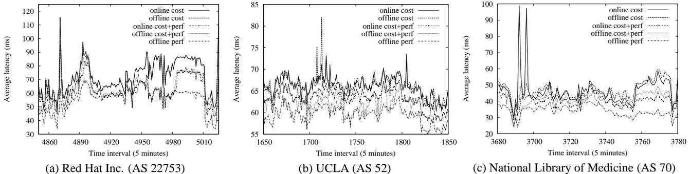
Figure 16: Performance comparison of different routing schemes.
