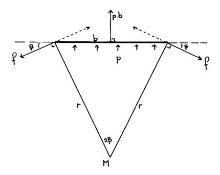
The outward force resulting from the pressure p exerted on a side of length b equals p.b and is applied to its midpoint in a direction orthogonal to it. The stability of the side requires that the parallel components of the two reaction forces cancel, and that their orthogonal components be p.b/2. Hence the two reaction forces have the same value, f say, and make the same angle,  $\beta$  say, with the side, the four quantities being related by p.b = 2.f.sin( $\beta$ ).
