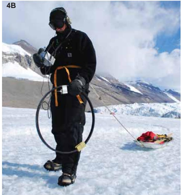
Figure 4: Emergency Recovery Beacon: 4A) onboard magnetic field generator; 4B) surface tracker in use on WLB
