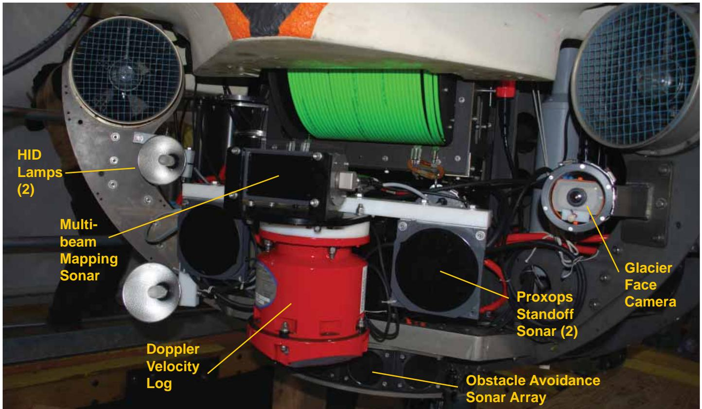
**Figure 9:** Glacier mapping and imaging array
