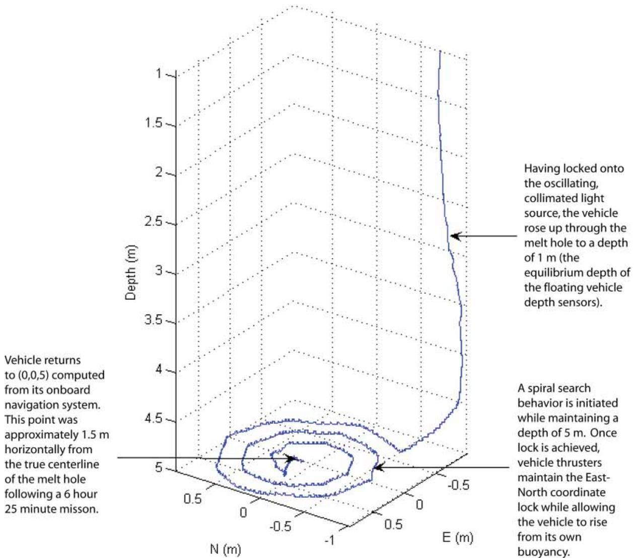
Figure 6: MatLab 3D plot of the auto-return-to-melt-hole system system in action during Mission 5. Coordinates are vehicle-centric (where the vehicle believes it is located relative to its initial starting position, including error) while the overhead collimated light oscillator represents the true centerline of the melt hole.
