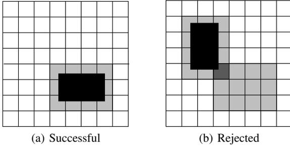
Figure 2: (a) The vehicle’s space-time request has no conflicts at time  $t$ . (b) The black vehicle’s request is rejected because at time  $t$  of its simulated trajectory, the vehicle requires a tile already reserved by another vehicle. The shaded area represents the *static buffer* of the vehicle.
