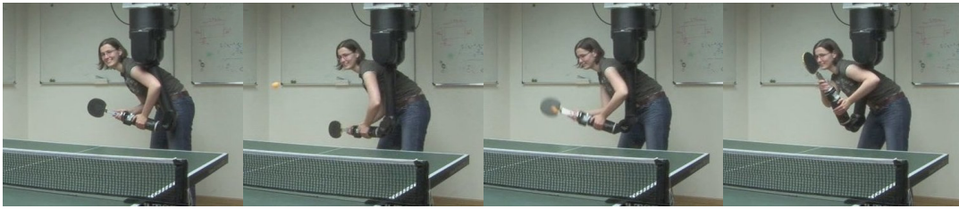
(a) Physical human robot interaction: kinesthetic teach-in of a striking motion in table tennis.
