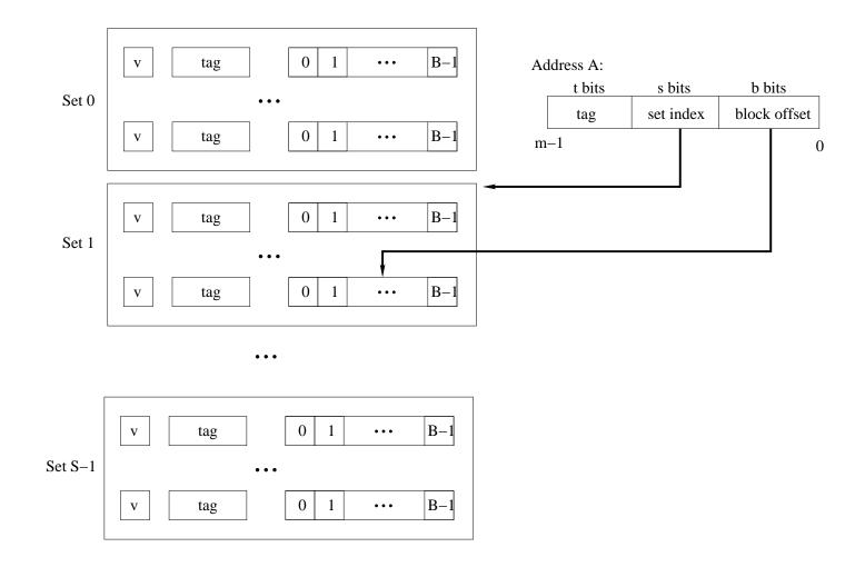
The word at address A is in the cache if the tag bits in one of the *valid* lines in set *set\_index* match *tag* for that line.
