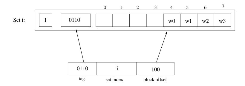
Suppose that the set index is 4 bits. What are the characteristics of this cache?
