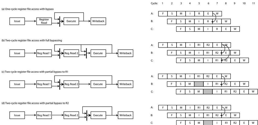
Figure 1: Different bypass implementations
