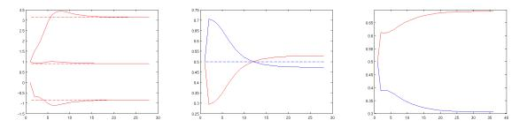
The left figure shows the convergence of the 3 covariance matrix entries to their real values. The other two figures shows the convergence of the  $\phi$  values (the probabilities of choosing Gaussian1 or Gaussian2 while generating data) to their values, in case they are both 0.5 (middle) and in case they are 0.3 and 0.7 (right).
