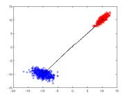
**Significantly overlapping Gaussians: classification depends on initialization** Here I generated two highly overlapping Gaussians. In the first experiment I initialized the means far from each other, on the boundaries of data, and in the second one I initialized both of them close to the center of data at two different points (Please zoom-in to see the details).
