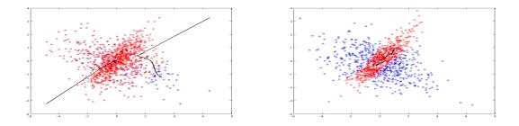
We see that here, initializing the means far from each other (left figure) didn't help to achieve convergence: after 131 iterations it converged to 54% accuracy. On the other hand initializing the means close to each other (right figure), which is also close to their real values, achieved impressive results: 39 iterations and 79% accuracy on two highly overlapping Gaussians.
