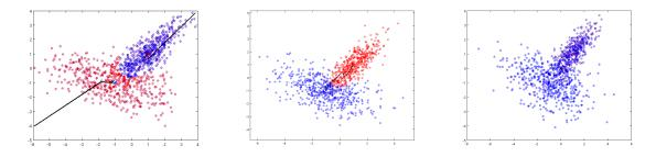
We see that when the means are initializing far from each other (left), or even close but not identically initialized (middle), and even though the Gaussians overlap, the results are pretty good: in the left figure #iterations=28, accuracy=93.5% and in the middle #iterations=32, accuracy=91.3%. However, on the right one, where the two means where initialized identically, all the points were assigned to the same cluster, achieving a baseline (bad) accuracy of around 50% (already a local maximum).
