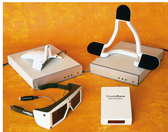
FIGURE 2-23 An ultrasound tracking device used with stereoscopic glasses to record changes in a viewer's head position. (Courtesy of StereoGraphics Corporation.)
