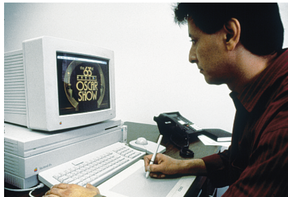
FIGURE 2-48 An artist's digitizer system, with a pressure-sensitive, cordless stylus. (Courtesy of Wacom Technology Corporation.)
