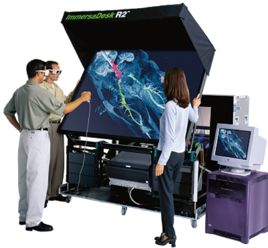
FIGURE 2-33 The SGI Reality Center 2000D, featuring an ImmersaDesk R2 and displaying a large-screen stereoscopic view of pressure contours in a vascular blood-flow simulation superimposed on a volume-rendered anatomic data set. (Courtesy of Silicon Graphics, Inc. and Professor Charles Taylor, Stanford University. © 2003 SGI. All rights reserved.)
