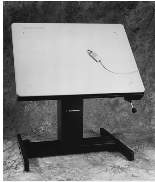
FIGURE 2-46 The Microgrid III tablet with a sixteen-button hand cursor, designed for digitizing larger drawings. (Courtesy of Summagraphics Corporation.)
