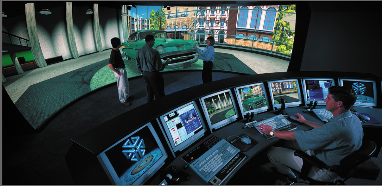
A wide, curved-screen, computer-graphics presentation system and its control desk. (Courtesy of Silicon Graphics, Inc. and Trimension Systems. © 2003 SGI. All rights reserved.)
