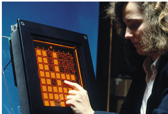
FIGURE 2-53 Plasma panels with touch screens. (Courtesy of Photonics Systems.)
