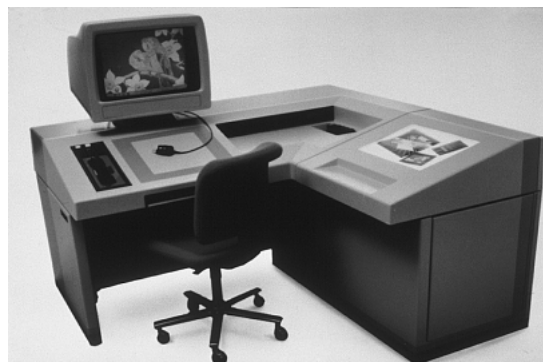
FIGURE 2-31 An artist's workstation, featuring a monitor, a keyboard, a graphics tablet with a hand cursor, and a light table, in addition to data storage and telecommunications devices. (Courtesy of DICOMED Corporation.)
