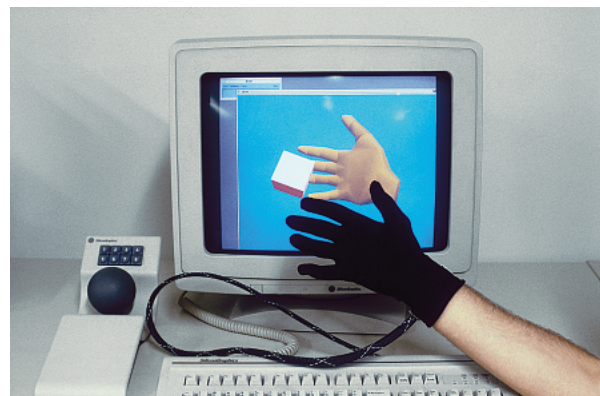
FIGURE 2-44 A virtual-reality scene, displayed on a two-dimensional video monitor, with input from a data glove and a spaceball. (Courtesy of The Computer Graphics Center, Darmstadt, Germany.)
