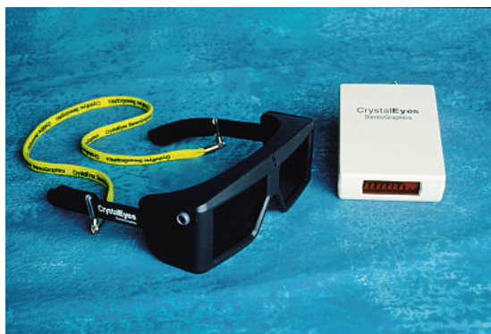
FIGURE 2-20 Glasses for viewing a stereoscopic scene and an infrared synchronizing emitter. (Courtesy of StereoGraphics Corporation.)
