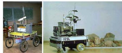
Left : The Stanford cart sports a single camera moving in discrete increments along a straight line and providing multiple snapshots of outdoor scenes Right : The INRIA mobile robot uses three cameras to map its environment
