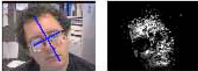
Figure 7: Orientation of the flesh probability distribution marked on the source video image
