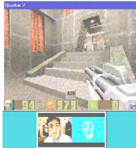
Figure 12: CAMSHIFT-based face tracker used to play Quake 2 hands free by inserting control variables into the mouse queue
