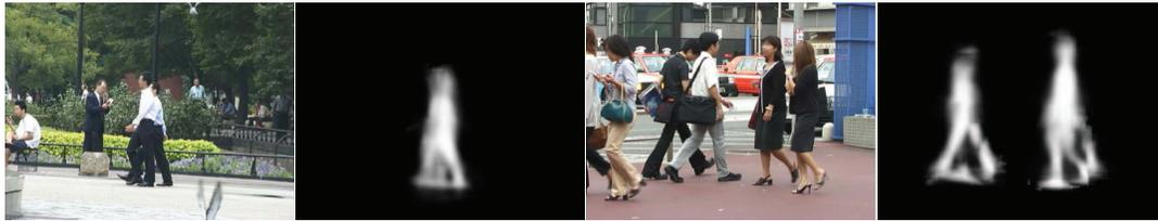
Figure 7.11: An important restriction of the star topology model used in the ISM is that no higher-level spatial relations between features are encoded. Each local feature that is consistent with the same object center may contribute to a hypothesis. For articulated objects, this may lead to additional body parts being associated to an object hypothesis (Figure from [LSS05]).
