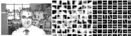
Fig. 3. Points of interest (left) identified on a training image of a human face in cluttered background using Forstner's method. Crosses denote corner-type patterns while circles mark circle-type patterns. A sample of the patterns obtained using k-means clustering of small image patches is shown for faces (center) and cars (right). The car images were high-pass filtered before the part selection process. The total number of patterns selected were 81 for faces and 80 for cars.
