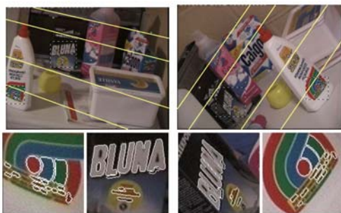
Figure 3: WASH: Epipolar geometry and dense matched regions with fully affine distortion.
