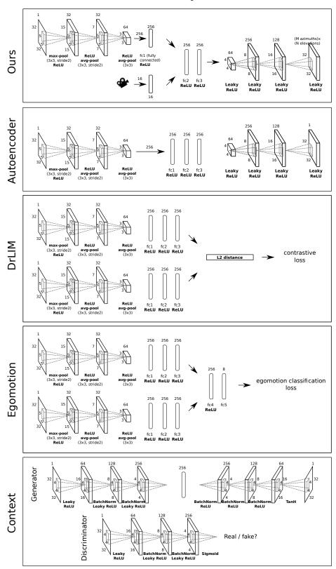
Figure 1: Architecture of our system and various baselines. See Sec 1.
