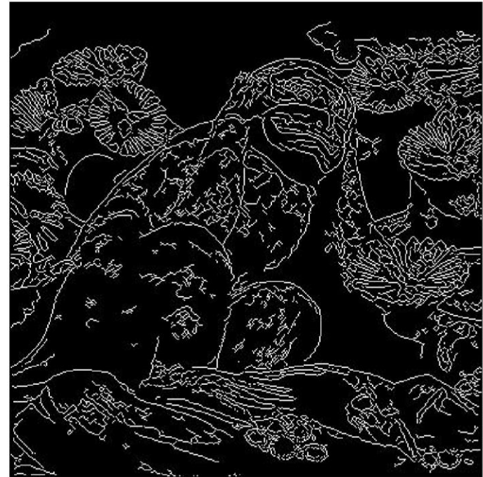
Figure 4.5. Edge pixels from the Canny edge detectors.
