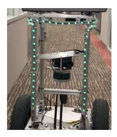
Above: Low light intensity levels indicate reduced speed of the BWI robot.
