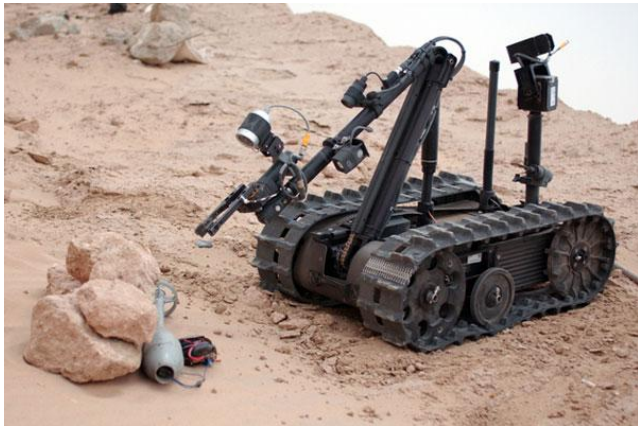
Figure 2: Unmanned, military scouting robot that has an arm and a camera to navigate its surroundings.
