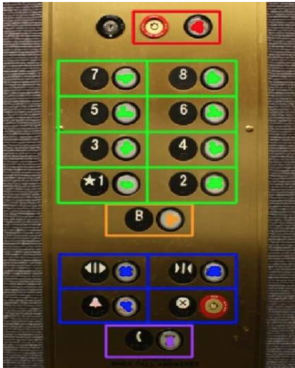
Fig (c) A picture of a robot using a red pointer to mark its desired point of contact with the button. Fig (d) The buttons are divided into grids and the center of each button is marked.
