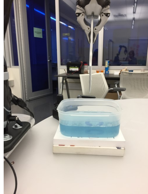
Figure 6: Image of the height adjustments required for trials with shorter stirrers. Pictured is the shampoo run with the plastic spatula; two books were used to raise the container.
