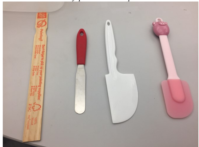
Figure 5: The stirring implements used for the trials, from left to right: wooden paint stirrer, metal icing spreader, plastic spatula and soft plastic/silicone spatula
