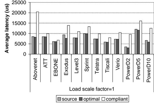
**Figure 3: User latency for all topologies with the  $M/M/1$  latency function and load scale factor 1. Selfish stands for selfish source routing; optimal stands for optimal routing; compliant stands for optimized-compliant OSPF routing. The other figures in this section use the same notation.**
