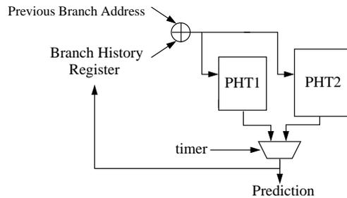
Figure 4.3: Cascading branch predictor
