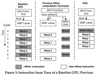
Figure 3: Instruction Issue Trace of a Baseline GPU, Previous Affine Computation Technique, and DAC.
