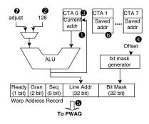
Figure 11: Address Expansion Unit
