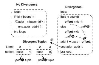
Figure 14: Divergent Base-Offset Pairs on SIMT Lanes
