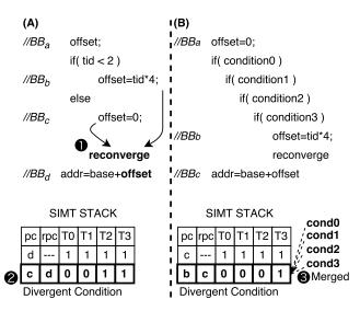
Figure 15: Using SIMT Entry as Divergent Condition
