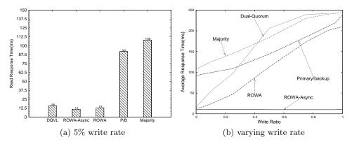
Fig. 6. Response time vs. write rate
