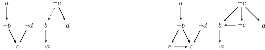
Fig. 4. \text{BIG}(F) in Example 6 before (left) and after (right) applying NHBR on F . Both graphs have three leaves: \neg a, c , and d . The dotted edge \neg c \rightarrow b is not in the in-tree decomposition.
