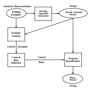
Figure 1: The CHILL Architecture
