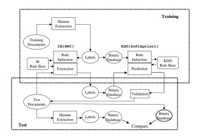
Figure 4: The system architecture
