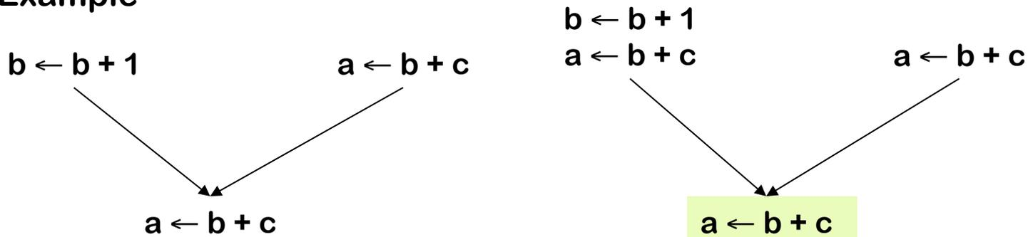
Inserting a copy of “ $a \leftarrow b + c$ ” after the definition of  $b$  can make it redundant
