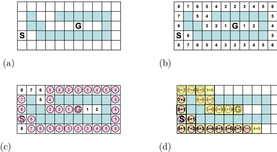
Figure 4: (a) An example of a search problem where the goal is to get from  $S$  to  $G$ . (b) The search space, labeled with the Manhattan distance heuristic. (c) The set of nodes expanded by best-first search. The solution is clearly suboptimal. (d) The set of nodes expanded by  $A^*$  search. (Note: the pair of numbers in each square represent the heuristic value  $h(n)$  and the distance already traveled  $g(n)$ .)
