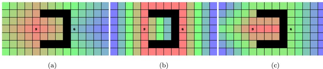
Figure 6: Some examples of the value of  $f(n)$  for different nodes during  $A^*$  search, when different heuristic functions are used. The value of  $f(n)$  is shown via a colorscale, where small values are red, intermediate values are green, and large values are purple. (a)  $h(n) = 0$ , e.g. blind search. (b)  $h(n) = h^*(n)$ . (c) Manhattan distance.
