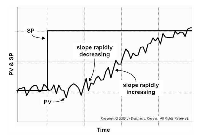
This is a problem if control output (CO) depends on slope (with a high gain).
