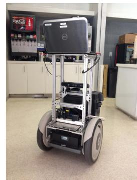
**Figure 4:** Robot platform (SegBot) used in experiments.
